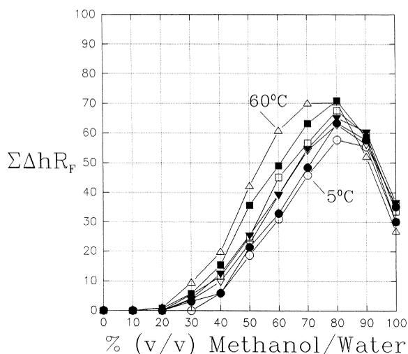
Fig. 3. Relationships between  $\Sigma \Delta hR_F$  values and composition of mobile phases at different temperatures, obtained for mixtures consisting of eight steroids. 5°C (○), 10°C (●), 20°C (▽), 30°C (▼), 40°C (□), 50°C (■), 60°C (△).
